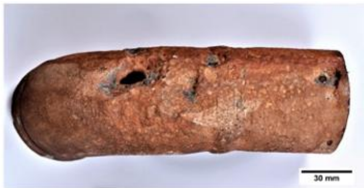
Figure 8: Large pits and perforations were seen on the surface of a steel pipe elbow.
